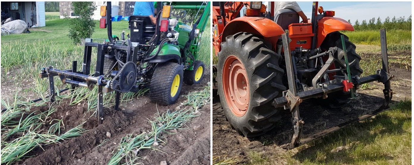
A small undercutter pulled by a 25 horsepower tractor (left) and a large undercutter pulled by a 55 hp tractor (right).
