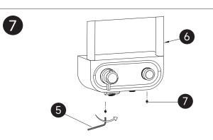
Screw the (7)hexagon screw into the (6) mixer with (5)hexagon wrench and tighten.
