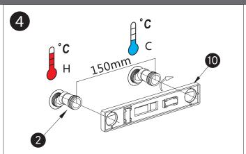
Level the product with (10) leveling instrument and adjust the centre distance of the (2)water inlet to 150mm.
