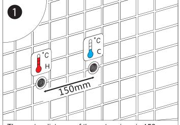
The centre distance of the water pipes is 150mm. The G1/2 outlets are on a parallel line.
