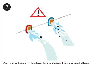
Remove foreign bodies from pipes before installing products. The installation of pipes must follow: hot on the left and cold on the right.
