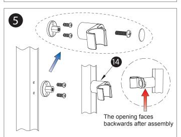
Loosen the screws of the (14) hand shower bracket. Place the (14) loose fittings over the two holes in the main body and screw them. Put the kit for the (14) hand shower bracket onto the fixed fitting and lock it with screws, then place the small cover.
