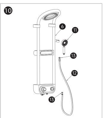
Place (13)rubber gasket into one (12) hose end and screw it to joint of the (6) mixer bottom. Screw the other hose end to (11) hand shower.
