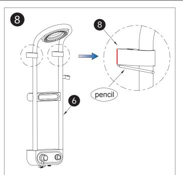
Level the (6) main body against the wall, insert the (8) bracket basement into the outer basement, place the (10) levelling instrument on the shelf to keep the (6) body level and mark on the (8) bracket basement with a pencil.
