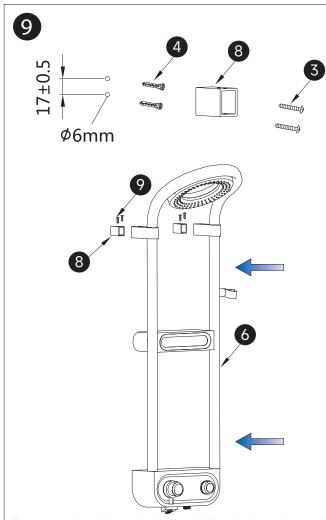
Remove the (6) main body, drill a hole in the wall at the marked position of the (8) bracket basement, hammer a (4) wall anchor into the hole and fix the (8) bracket basement with a (3) screw. Insert (6) main body into the (2) water inlet joint, insert the upper end into the secured (8) bracket basement and lock with (9) screws.
