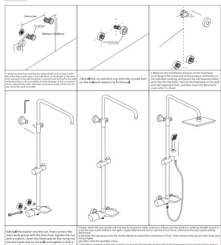
main body group with the bent foot, tighten the nut with a wrench, insert the fixed seat on the rising rod into the fixed seat on the wall, and tighten it with a hexagonal wrench after adjusting the position. If the position of the product is slightly out of alignment during installation, the partial bath pipe support car be adjusted appropriately.
