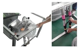
b. Place Cargo bike on a flat surface, take out the front fender and front wheel, then assemble them well. And then assemble the front brake cable.
