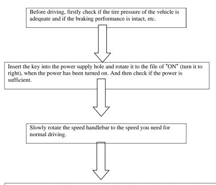
When you need parking, firstly rotate back the handlebar to decrease the speed, and then brake the tricycle, rotate the key to "OFF" and unplug the key.
