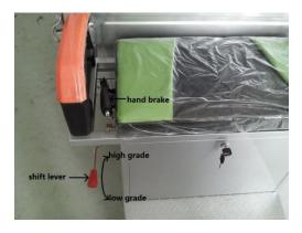
Note1: When changing the gears, you must stop the Cargo bike.
