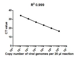
**PhoenixDx® qPCR Mastermix Bravo** was used for the detection of SARS-CoV-2 RNA using SARS-CoV-2 specific primers in a probe-based multiplex qPCR with the described 2-Step Standard protocol. The serial dilution of SARS-CoV-2 RNA was detected with a high linearity and less then 5 copies were detected in >95 % of replicas.
