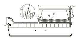
**Step 8**Hang the main grill (29) in the lifting system iron wire. Put the three separate grill (20) in the main grill frame (29).
