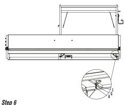
Fix the elevation system in the main body using M6\*12 screws (A), M6 spring washers (G) and D6 washers (1).
