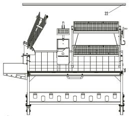
**Step 15**Place the trash block bar (22) on the mainbody next to the front door.
