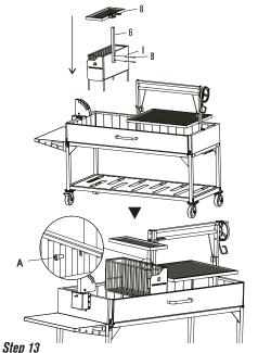
Place the brazier (5) beside the main grate. Fix the support bar (6) using M6\*40mm hexagon screws (B) and D6 washers (I). Insert the secondary grate (8) into the assembled support bar (6), and fix it using the ring screw (M). Screw the brazier with left rod of lifting system.
