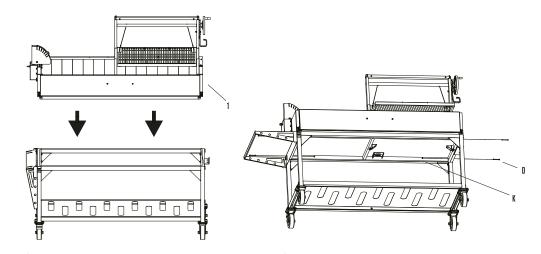
Step 9 First, make sure to lock the wheels to leave the base on its place. Carefully place the main body (1) on the lower structure.
