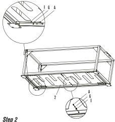
Assemble the two sets of legs with the bottom shelf (2) using M6\*12mm hexagon screws (A), D6 washers (I) and M6 spring washers (6) inside.
