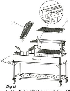
Insert the grilling basket (13) into the clamp grille basement. Place the top warming rack on the top of elevation system top bar, fix it using M6\*12mm hexagon screws (A).
