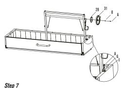
Insert the gear (28) and wheel in the lifting rod. Fix them using the D6\*20 washer (0) and a M6\*12 hexagon screw (A). Fix them on the main body using two M6\*12 hexagon screw (A) and M6 spring washers (G) and D6 washers (I).
