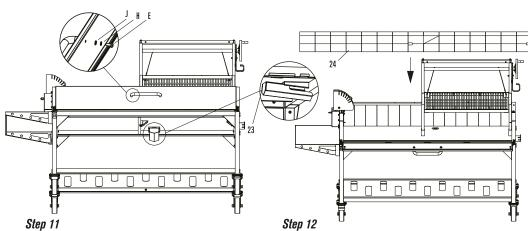
Place the firebricks (24) into the body. The firebrick with chipped Assemble the handle (21) in the front door using M8\*16 screws (E), M8 spring washers (H) and D8 washers (J). Slide the water corner goes first around the square tube. We recommend to even drain (23) under the drain hole. out the space between the firebricks before the first use with a knife or screwdriver.
