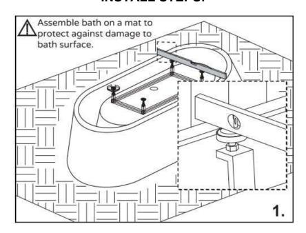
• Ensure legs are adjusted in line with the base of bath.
