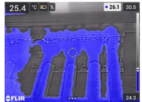
Below alarm: Highlights all pixels with a temperature below the specified temperature level.
