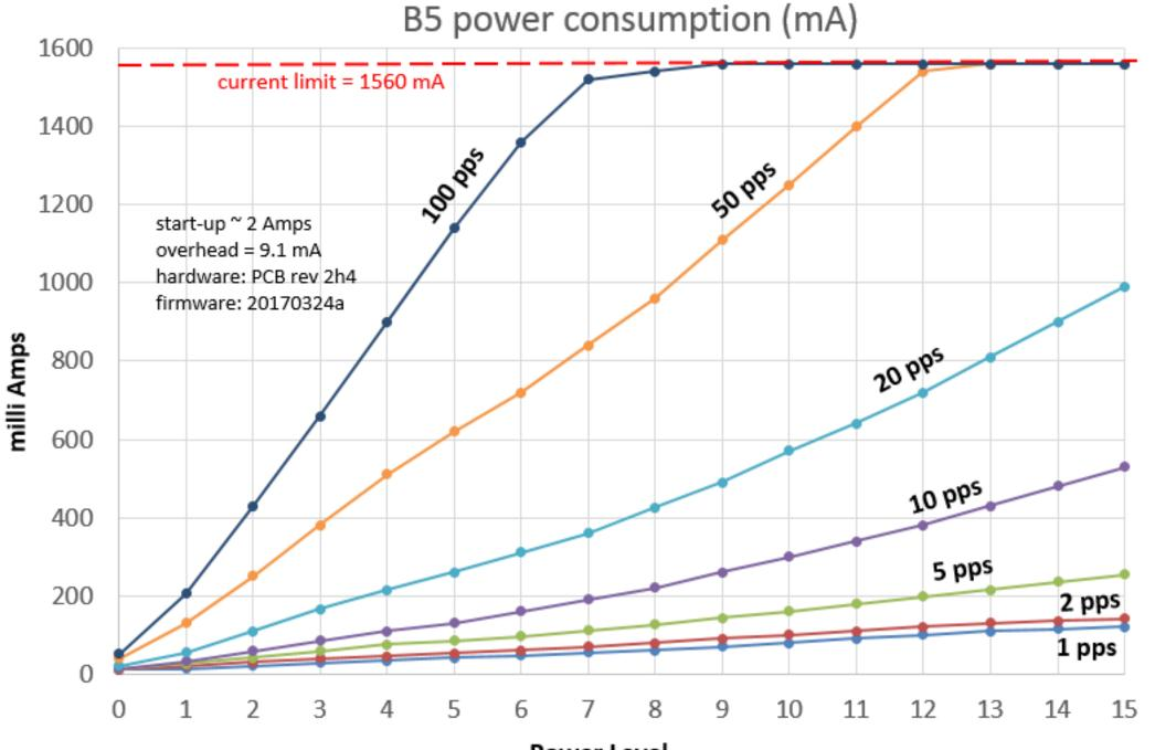
It will continue at the high on POWER-UP, it will reset You can increase it again manually. if current limit is exceeded, the RED LED will light for  $^\sim 1$ B5 will resume function. set, but next time, s safe level, usually POWER = power level you have second, then the NOTE:
