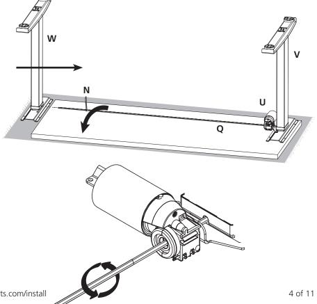
• Tighten motor mounting bolts after hex rod is installed.
