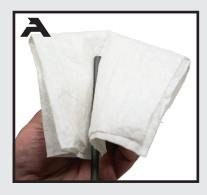
**Clean the outside** of the shaft with alcohol to remove any residue.
