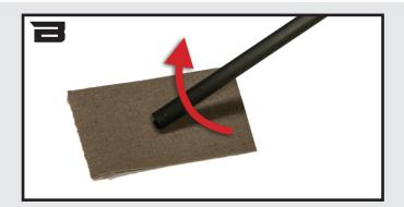
Lightly chamfer the edge of the carbon arrow to eliminate any flaring that may have occurred during cutting/squaring process. This can be done by placing a 320 grit or higher piece of sandpaper on a flat surface, holding the arrow at a slight angle, and lightly rotating the front edge of the arrow shaft on the sandpaper.
