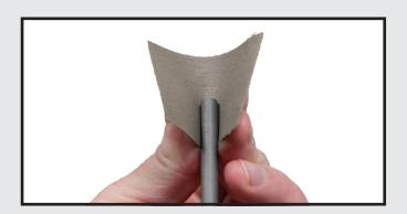
**Lightly sand the first ½"** of the shaft using a 320 grit or higher sandpaper or Scotch Brite pad by wrapping the end of the arrow shaft with the sandpaper or pad, applying light pressure then rotate the shaft. Be careful not to sand too much as this could leave the outsert with a very loose fit. The shaft should be sanded with light pressure and should be cleaned and checked often through this process to dial in the outsert fit.
