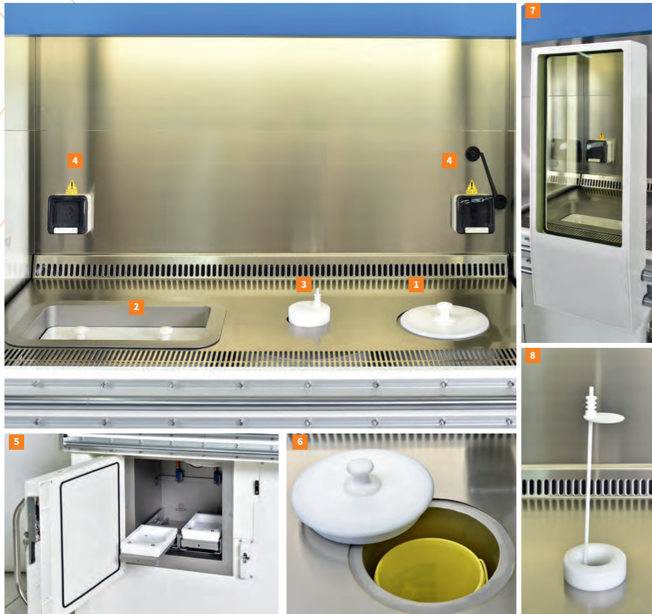
1 | 1 waste bin 2 | 2 independent accesses for each generator 3 | 1 access for the dose calibrator 4 | 2 socket emplacements (electrical, USB, RJ45) 5 | 1 shielded lockable compartment for 2 generators, equipped with 2 loading trays and 2 independent lifts 6 | Access to the waste compartment from the work surface 7 | Sliding, removable and retractable lead glass screen 8 | Posilift system (raising and lowering of the dose calibrator dipper by foot control)
