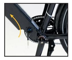
Push the battery all the way into the downtube and lock the battery by turning the key to the right. You can only remove the key if the battery is properly mounted and locked in place.
