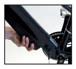
Support the battery with one hand, then remove it from the frame by turning the key left and pushing the battery up and pulling down. The battery is a snug fit, so if too tight to remove, a sharp tap on the side of the downtube with the heel of your free hand will help release it.
