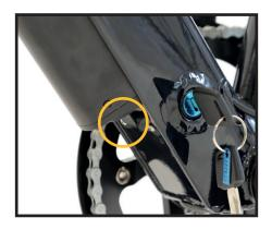
When the key is turned to the right, press the battery button that is highlighted on the photo to release the battery.
