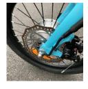
Loosen the cable clamp at the brake caliper. Position the cable in the cable clamp. Tighten the cable clamp (particular attention should be paid to each end of the sheath which must enter without forcing into the housing of each rigid end piece, on the brake handle side).
