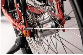
Detach the cable from its housing Detach the sheath stopper from the hub by turning the cable 90°
