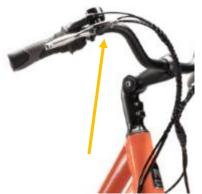
Loosen the cable clamp and pull the cable until the pads contact the rim. Tighten the cable clamp (particular attention should be paid to each end of the sheath which must enter without forcing into the housing of each rigid end piece, on the brake handle and V-Brake side.)
