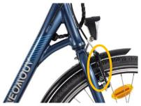
The pads are properly adjusted when they are an equal distance from the rim. The final adjustment is to be made by tightening the screws mounted on the pad supports with a Phillips screwdriver (distance of approximately 0.1 to 0.5 mm from the rim).
