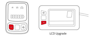
For bikes with a throttle, the red button is depressed and the throttle grip twisted to activate. For safety, when not in use ensure the red button is left out to avoid accidental use of the throttle.
