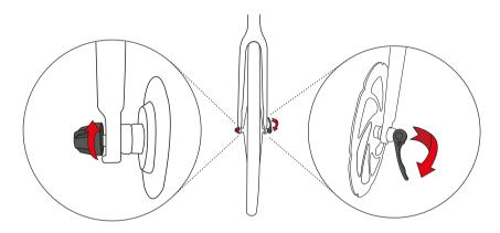
With the lever open, the  $\underline{nut}$  is used to both loosen and pre-tighten the mechanism.
