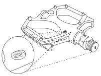
Using finger & thumb (and later a 15mm spanner) attach the pedals onto their crank arms. The R pedal will be tightened in a **clockwise** direction.
