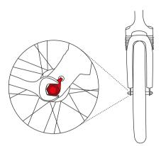
Our Compact bike front wheel is fitted with a standard nut and locating washer. Making sure the small washer locates into the forks, tighten using a 15mm spanner and again be sure to always check the wheel runs true, centred within the forks.
