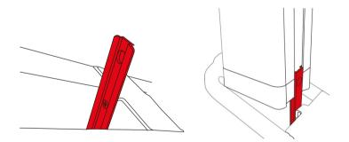
Once fully inserted, turn the key **clockwise** into the **OFF** position to lock the battery in place. The key can then be removed.
