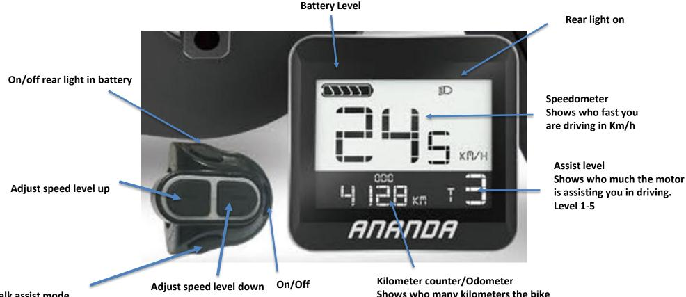
Walk assist mode Activates PAS-walk/Walk-assist function Hold down for 2 sec, and the bike will drive on its own, stops when button is released
