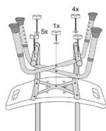
5. Screw the seat tubes and the seat together with a short wing screw and a washer
