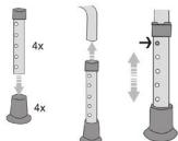
1. Fit the rubber feet on the foot tubes
