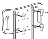
6. Place the back rest tubes 8 on the seat tubes so that the screw holes are aligned above one another.
