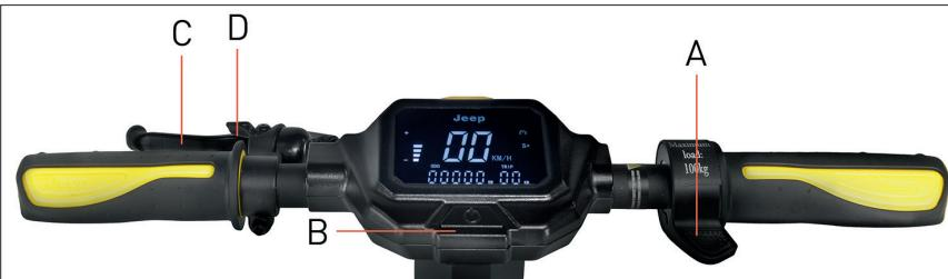
Throttle (A): press down to accelerate.
