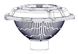
Dimensions Float width w/ brackets: 28" Unit height with float: 18"
