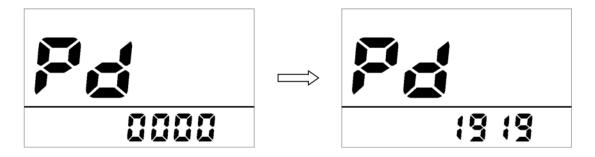
3. Single Press "M" to enter the following interface, press "+" to change to any number above 20mph. Long press "M" to save your settings. The max speed is now 25mph.
