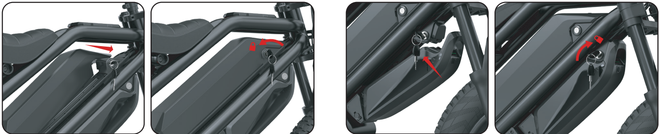
GT version battery installation
