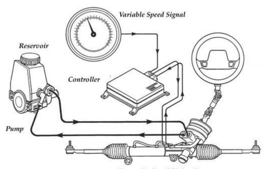
Power Rack and Pinion Gear
