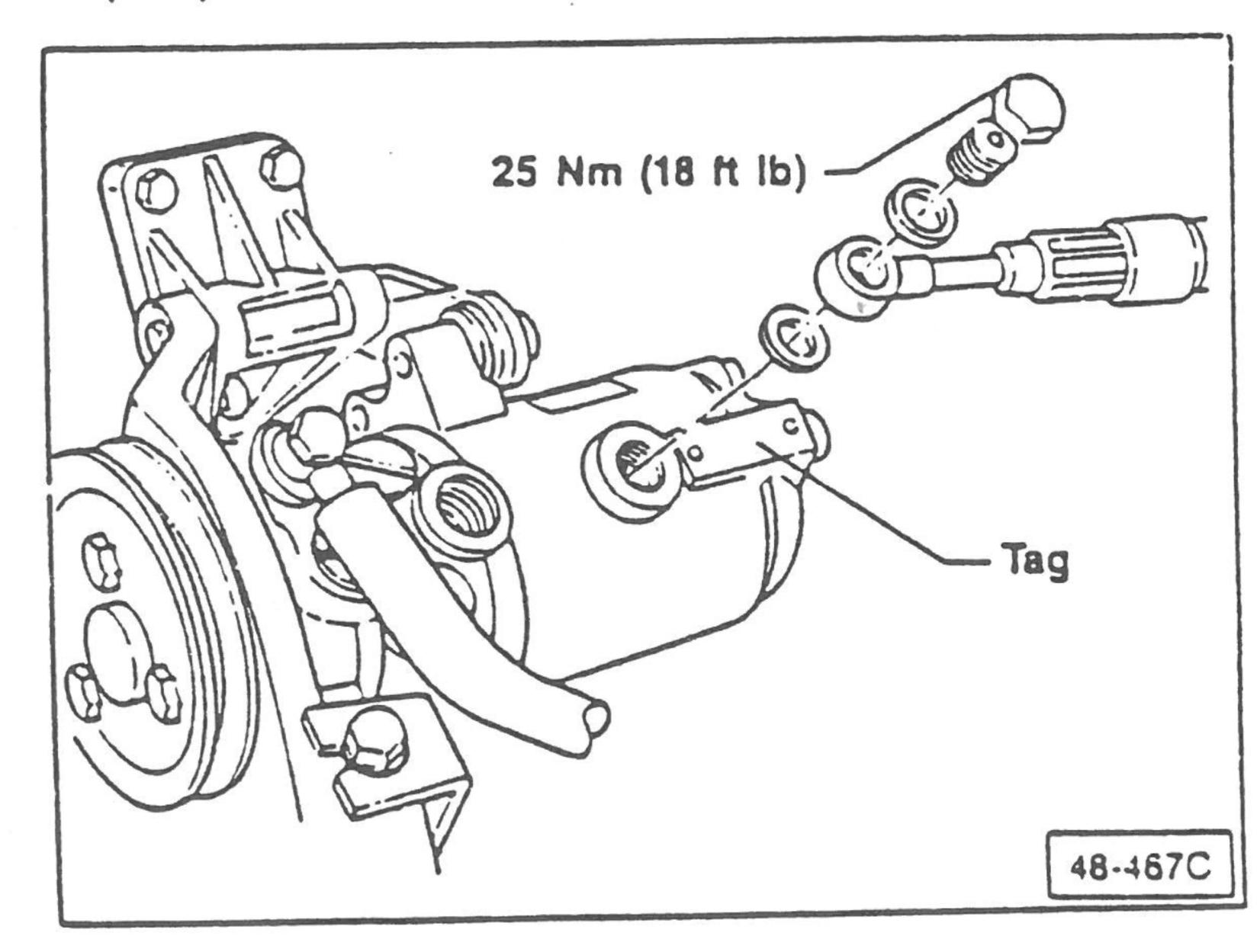
— connect pressure line to pump using correct banjo bolt:
