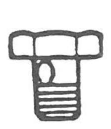
— connect suction line to pump using correct banjo bolt:
