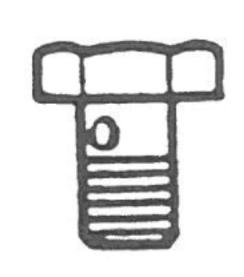
• pump with silver tag: use banjo bolt with three large holes and no screen Part No. N 021 071 2
