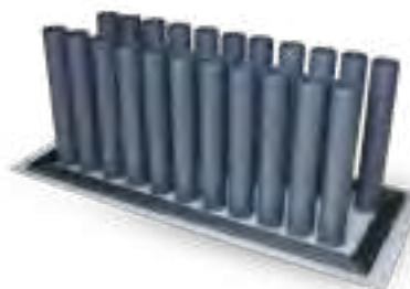
KRASO® Multi System Penetration Type FE 2 x 11 - Special plate size approx. 1495 x 590 mm, incl. 22 casings ID 80, water pressure tight surrounding KRASO® 4 Seal on the plate and surrounding trowel flange roughened, wall thickness approx. 560 mm
