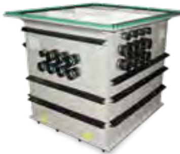
KRASO® Pump Sump Type Q - Special with 15 cm surrounding fixed-flange and water pressure tight surrounding KRASO® 4 Seal on the fixed-flange, reinforcing ribs and concrete anchors and 35 water pressure tight KG pipe connections internal dimensions: approx. 145 x 170 x 135 cm total weight: approx. 290 kg
