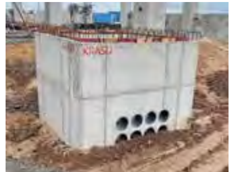
KRASO® Pump Sump - concrete - Special internal dimensions approx. 160 x 160 x 1,95 cm, 8 KRASO® Casings Type FE ID 200, made of waterproof concrete, with 20 cm thick, reinforced wall and base plate (20 kg per cbm ). rebar connection approx. 8/15 two-rowed, surrounding water pressure tight, MPA-tested construction joint tape KRASOflex® Duo-Fix 150 „plus“, 4 lifting lugs Rd30, total weight: approx. 8.80 t
