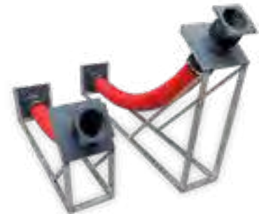
KRASO® Cable Inlet Box System KDS 150 - Special bending radius approx. 200 cm, for the secure connection of supply lines such as e.g. water - electricity - telecommunication etc. in buildings without basement. With installation device, empty pipe insert 20 cm and water pressure tight surrounding KRASO® 4 Seal and 2 KRASO® KDS Closure Covers
