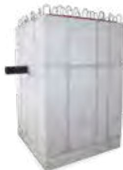
KRASO® Pump Sump - concrete - Special internal dimensions approx. 104 x 104 x 192 cm, made of waterproof concrete, with 20 cm thick, reinforced wall and base plate (20 kg per cbm), rebar connection approx. 8/15 two-rowed, water pressure tight surrounding, MPA-tested construction joint tape KRASOflex® Duo-Fix 150 „plus“, incl. PE pipe DN 124 with water pressure tight surrounding KRASO® 4 Seal with protrusion on both sides approx. 15 cm, 4 lifting lugs Rd20, total weight: approx. 5.94 t
