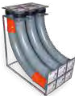
KRASO® Cable Inlet Box System KDS 150 - 2x3 - Special with water pressure tight surrounding KRASO® 4 Seal , suitable KRASO® KDS empty pipe insert 20 cm, 90° empty pipe system, installation device and 12 KRASO® KDS 150 Closure Covers
