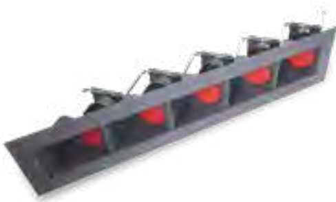
KRASO® Cable Penetration 150 - package 1x5 - as oblique double wall penetration at 45 degrees - incl. surrounding roughened trowel flange at one side - Special for the horizontal installation of supply lines at 45° angle, such as e.g. water - electricity - telecommunication etc. in buildings with a basement, with water pressure tight surrounding KRASO® 4 Seal , with roughened trowel flange
