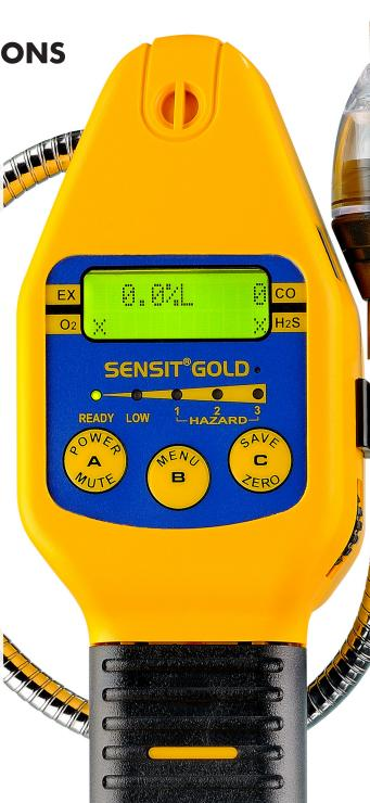
7. Extend the goose neck (the LEL sensor and filter cap is at the tip).
