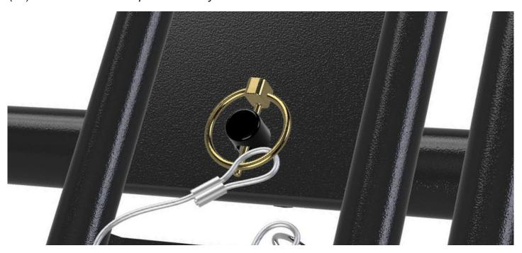
To secure the loading ramp, tether the lanyard to the loading ramp with the supplied key ring, insert linch pin through the receiver post and then fold down the snap ring.
