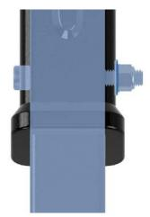
Do NOT put a washer on the head of the bolt - the washer goes on the nut end. Insert the bolt into the hitch pin hole and ensure the bolt head recesses into the hitch pin hole until it stops against the MotoTote tube inside the hitch. This is critical to eliminating any shake by clamping the square tube to the hitch. Then using an allen wrench and a socket wrench, tighten until the connection to the hitch is solid with no play. Do not over-tighten.
