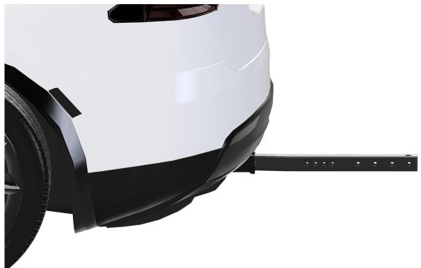
To start assembly, insert the square tube several inches into the hitch. This will make things easier by getting the carrier off the ground at a more comfortable height for assembly. You'll see more details about the ZeroWobble Hitch Mount when you get to <u>Step 5</u>.
