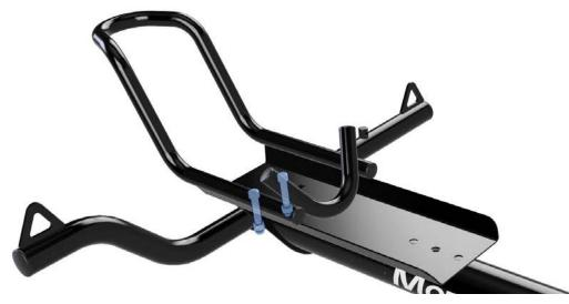
Place the front tie down arm in the slot of the platform, making sure the curved section if facing outward. Lay down the the wheelstop onto the platform and align with the holes then insert two bolts to the desired placement (there are three positions dependent on your motorcycle length). Put on the nuts and hand tighten only for now (this is to ensure alignment of loading ramp in Step 4).
