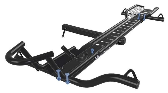
Now, tighten the nuts that you previously hand tightened onto the two bolts under the front wheelstop. Tighten all nuts and bolts snugly to minimize rattling - Do not over tighten. NOTE: Max+ parts shown but procedure is the same for Max & m3.
