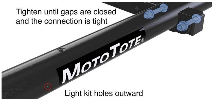
Slide the MTX platform onto the square tube aligning the holes. Find the two big hex head bolts, two nuts, and four washers. Slide one washer on the bolt and guide through the platform. Place washer on the other side and secure with a nut. Repeat process on both sides.(Note: If you plan to use the optional LED Light kit, attach the MTX platform so the holes are facing rearward)
