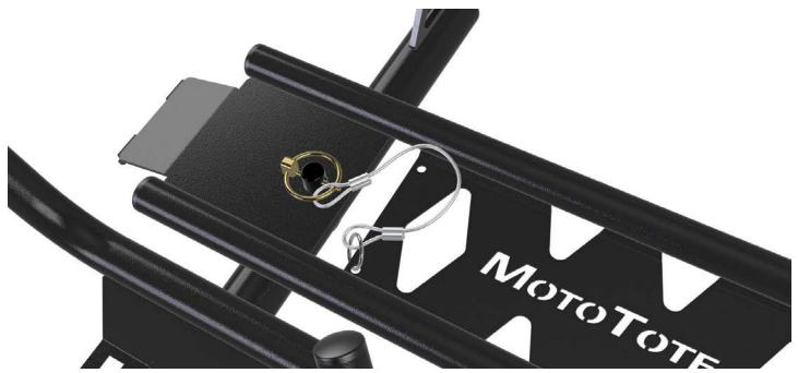
To secure the loading ramp, tether the lanyard to the loading ramp with the supplied key ring, insert linch pin through the receiver post and then fold down the snap ring.
