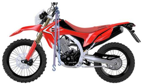
Prior to loading the bike, make a plan for your tie downs. It is important that they are easily accesible once the bike is up the ramp. For bikes with large fenders, we recommend attaching the tie downs to your planned location on the handlebars before loading. For other bikes, we recommend attaching the tie downs to the loops on the MotoTote first, then pulling up and securing the tie downs once loaded. Try both to find your preference.
