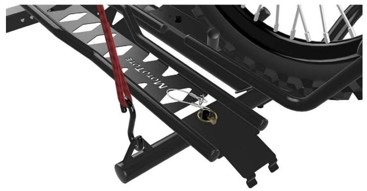
Lift and detach the loading ramp from the tire track. Place in dedicated position on ramp keeper tab and linch pin reciever post. Insert linch pin and flip to secure. Double check your work! The likliest mishap is a tie down error. You are now ready to roll!
