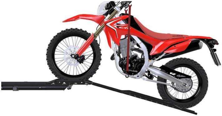
Tilt the bike toward yourself and lean into it, using your body weight to help push the bike up the ramp until you roll into the front wheelstop. Some users prefer to get a rolling start before pushing the bike up the ramp.
