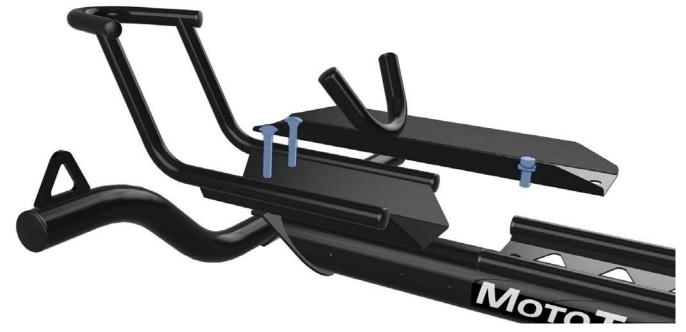
Place the front tie down arm in the slot of the platform, making sure the curved section is facing outward. Lay down the two parts of the wheelstop (front stop & back stop) onto the platform, align the holes to the desired placement, then insert two bolts. Put on the nuts and washers then hand tighten only for now (this is to ensure alignment of loading ramp in Step 4). Then put short bolt with the lockwasher through the back stop and tire track into the threaded hole on the platform tube.
