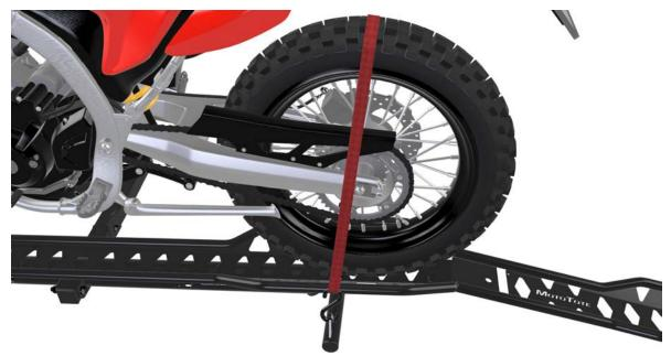
With a single tie down or an AceBikes Tyrefix, tie the strap directly over the back tire and tighten. The main objective here is to keep the rear tire from bouncing out of the track. For a scooter you can go over the seat or luggage rack.
