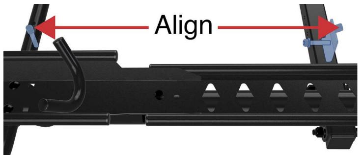
First make sure the angled flap of the tab is pointing toward the back end of the tire track, then place the ramp tab in line with the linch pin receiver post on the front tie down arm. Secure with a bolt, washer and nut. Tighten in place.
