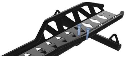
Now, on the opposite side of where you selected to put the wheelstop, insert the rear tie down arm into the slot and lay down the tire track on the platform. align with the two holes. Insert the two bolts into the tire track and through the holes. Put on the nuts and washers then tighten snugly to minimize rattling Do not overtighten. NOTE: The tracks look different but procedure is the same.
