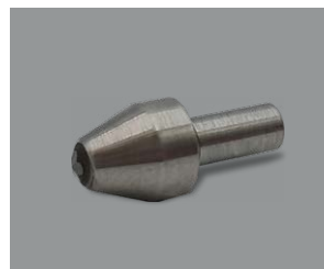
ISO/DaKKS Certificated Vickers and Knoop Indenters
