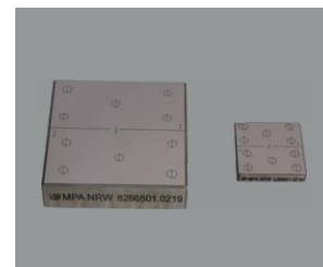
ISO/DaKKS Certificated Test Blocks
