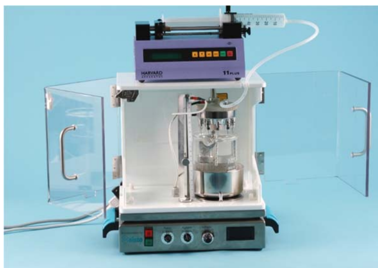
Fig. 4.3.3.1: Encapsulation unit VARV1 with 10 nozzles head
