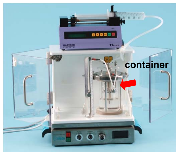
Fig. 4.3.4.2: Encapsulation unit VARV1 with sterile autoclavable container
