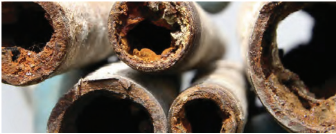
Scale buildup in pipes without scale prevention
