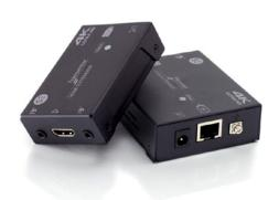
HD-EXR-100-HDBT is a 4K2K HDMI over HDBaseT extender kit (Tx/Rx) for HDMI transmission up to 100 meters (UHD resolution up to 70m) over a single CAT5e/CAT6/CAT6A cable with Bidirectional IR control capability. The kit is HDCP compliant and supports HDMI up to 10.2Gps, including support for 1080p 60, Deep Colour, HD-3D, 4Kx2K video, HD Audio Formats and Audio Return Channel. It only needs power supply at either Transmitter or Receiver end.
