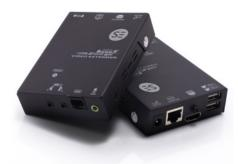
3D HDMI HDBaseT Extender transmits full uncompressed 3D UHD HDMI signal, 4 USB signals and independent audio (analog stereo and Toslink (SPDIF)) over CAT5e/6/6a cable of up to 100 meters. It supports UHD (3840 x 2160) up to 90 meters and Full HD (1920 x 1080) up to 100 meters.
