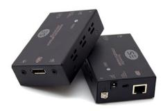
SEDG-DP100EXT is a DisplayPort over HDBaseT extender kit (Tx/Rx) for DisplayPort signal transmission up to 100 meters (WQXGA (2560 X 1600) resolution up to 70m) over a single CAT5e/ CAT6/CAT6A cable with Bi-directional IR control capability. The kit is HDCP compliant and only needs power supply at either Transmitter or Receiver end. EDID Migration ensures the optimum video performance and supports resolutions up to WQXGA (2560 X 1600) and Full HD 1080p
