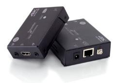
HD-EX-70-HDBT is a 4K2K HDMI over HDBaseT extender kit (Tx/Rx) for HDMI transmission up to 70 meters (UHD resolution up to 35m) over a single CAT5e/CAT6/CAT6A cable. The kit is HDCP compliant and supports HDMI up to 10.2Gps, including support for 1080p 60, Deep Colour, HD-3D, 4Kx2K video, HD Audio Formats and Audio Return Channel. It only needs power supply at either Transmitter or Receiver end.
