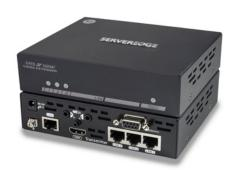
HDMI HDBaseT Extender over CAT5e/6/6a transmits uncompressed digital HDMI signal, Serial (RS232), IR, and Ethernet up to 100 metres over a single CAT5e/6/6A cable using HDBaseT technology. Each video extender consists of a local unit that connects to an HDMI source and a remote unit that connects to an HDMI display.
