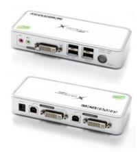
KD02UDH2 is a 2-port Slim Palmtop USB KVM Switch with audio and microphone switching function. It allows you to access, control, boot and reboot 2 DVI-enabled USB multimedia computers. The independent audio/mic switching function allows an uninterrupted audio experience on a same connected computer even when you switch to another computer.
