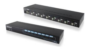
The KR08HHU is a rack mountable KVM switch with the HDMI video interface designed to control 8 PCs from a single keyboard, mouse and monitor console. It also provides support for multimedia keyboard, audio & mic. The KVM enables computer selection via both front panel push buttons & hotkeys. \*Cables required to connect the monitor and the computers are sold separately. Suitable Cables: HDMI-02-MM-V4, HDMI-03-MM-V4, USB2-02-AB, USB2-03-AB, MM-AD-02, MM-AD-02
