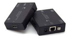
HD-EX-70-HDBT is a 4K2K HDMI over HDBaseT extender kit (Tx/Rx) for HDMI transmission up to 70 meters (UHD resolution up to 35m) over a single CAT5e/CAT6/CAT6A cable. The kit is HDCP compliant and supports HDMI up to 10.2Gps, including support for 1080p 60, Deep Colour, HD-3D, 4Kx2K video, HD Audio Formats and Audio Return Channel. It only needs power supply at either Transmitter or Receiver end.
