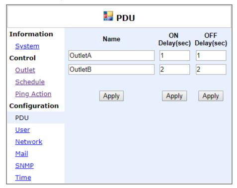
**Note**: After PDU is plugged into main power, PDU system will start to sequentially turn on the output socket according to the pre-set delay time in PDU web interface. The factory default setting for delay time is one second for each outlet; therefore the 8 ports PDU will take 8 seconds, 24 ports PDU will take 24 seconds to complete start-up procedure.
