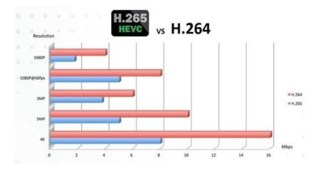
• **H.265** compression allow further reduce the network bandwidth consumptions in transmission and take up less storage space.
