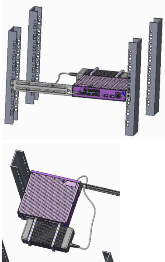
Figure 56: V300-8P-2X Single Rack Mounting with PSU
