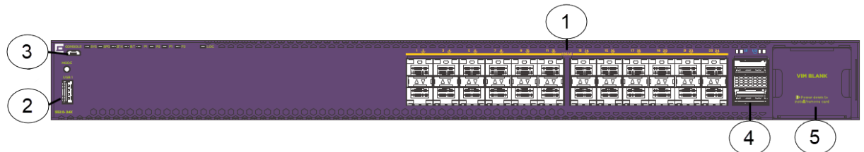
Figure 5: 5520-24X and 5520-24X-BASE Front Panel
