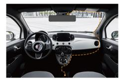
Step3: Connect the interface of the rear cable with the interface of the docking station, and hide the rear camera cable inside the vehicle.
