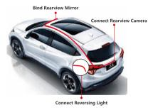
Note: If wiring doesn't meet expectations for installation in the vehicle, cable clips can be used to secure the cables installation as desired.
