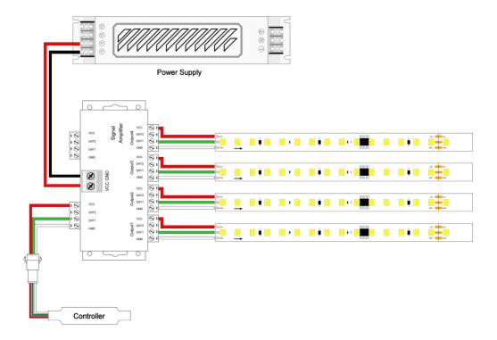
Connect the strip to the amplifier (please make sure to connect with correct wire, if there is connector on strip, just cut off connector), connect the controller to the amplifier, connect the power adapter to the amplifier. Power on and enjoy it.
