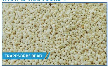
Each **Trappsorb**® bead is only a few microns across to be of use in fixed bed Adsorption process. It is necessary to form beads in the range of 1.2 - 3.4 mm in diameter. Within the above range a wide selection of **Trappsorb**® beads sizes can be produced to suit the specific needs of the customer.
