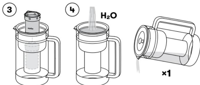
3. Place the filter cartridge in the hopper.
