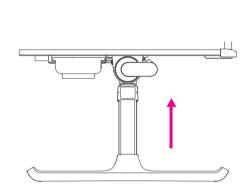
Pull up the table to the required height and it will be locked automatically.
