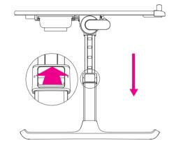
Press down the 2 lock buttons as illustrated and lower the table to the required height, then release the button and it will lock automatically.
