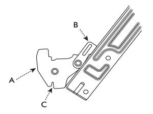
2. Lift up and turn the small levers (B) situated on the two hinges (A).
