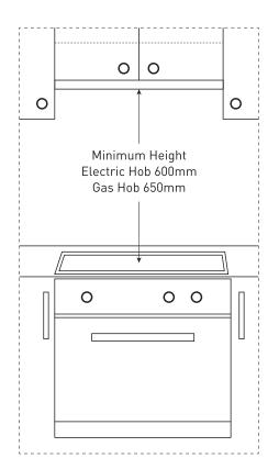
Fig 1.2 illustrates the minimum height from the hob surface to the underside of the rangehood. Electric hob – 600mm, Gas hob - 650mm.
