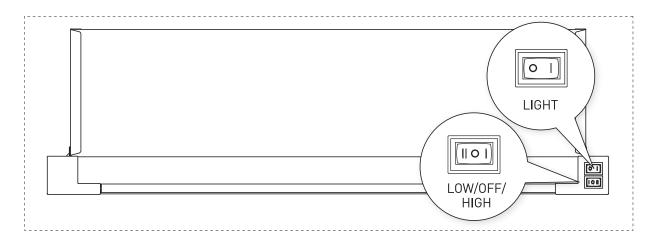
**IMPORTANT** // To operate the unit, ensure that the power is turned on and the front visor is fully extended. This will provide access to the light and speed controls.
