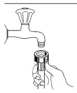
Connect the cold water supply hose to a threaded 3/4(inch) connector and make sure that it is fastened tightly in place. If the water pipes are new or have not been used for an extended period of time, let the water run to make sure that the water is clear and free of impurities. If this precaution is not taken, there is a risk that the water inlet can get blocked and damage the appliance.
