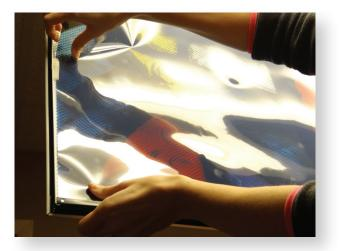
**Step 3:** Place your Apollo DesignScapes® artwork side down on top of the plastic diffuser cover. There is no need to remove the diffuser panel.
