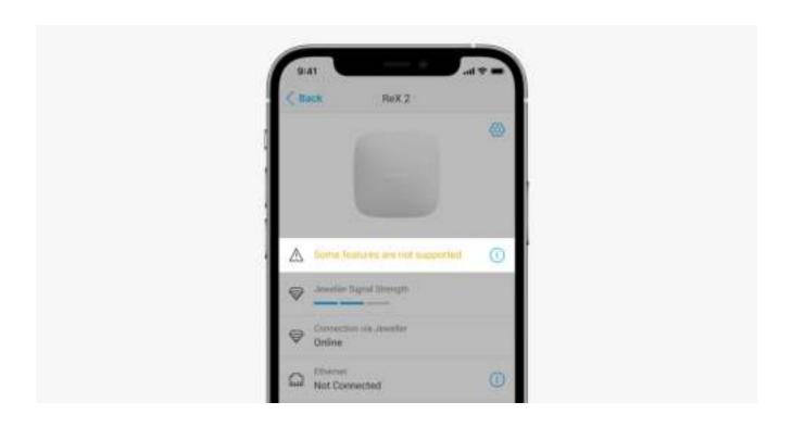
ReX 2 can notify about malfunctions, if any. **Malfunctions** field is available in **Device States**. Clicking on (i) opens the list of all malfunctions. The field is displayed if a malfunction is detected.
