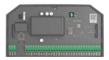
The MultiTransmitter LED indicator may light up in white, red, or green depending on the device status. Note that the LED indicator is not visible if the lid is closed,
