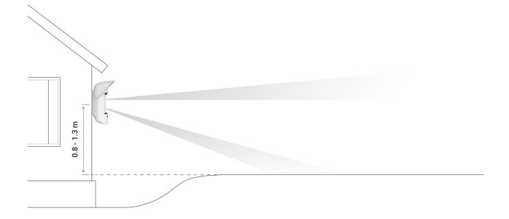
The detector can be placed 0.5 meters above ground level to protect the facility from crawling burglars. In this case of installation, the pet immunity function is not available. This mounting height of the detector is recommended for installation in industrial facilities and warehouses.
