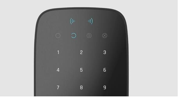
You can use the KeyPad Plus without ambient lighting as the keypad has a backlight. The pressing of the buttons is accompanied by a sound signal. The backlight brightness and keypad volume are adjustable in the settings. If you do not touch the keypad for 4 seconds, KeyPad Plus reduces the backlight brightness, and 8 seconds later goes into power-saving mode and turns off the display.
